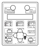
4. Press the [Cleaning] key on the operation panel for at least two seconds.
