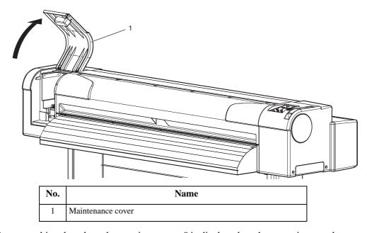
• "Remove white plate then close mainte. cover." is displayed on the operation panel.
