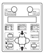
5. To save the changed setting, press the [Enter] key on the operation panel.
