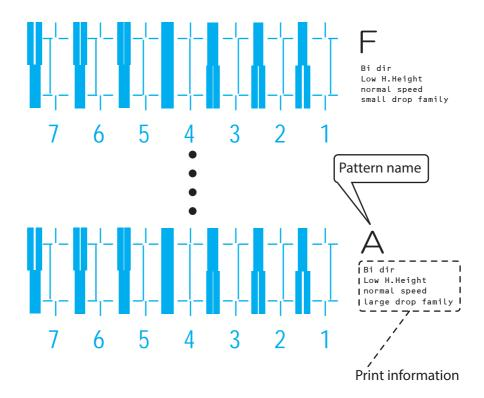
• For the Adjust print pattern, the same patterns will be printed repeatedly on both sides and center of the media.
