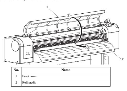
5. While holding the edge of the media, rewind the roll media a little by turning the scroller by hand and eliminate any slack or slant.
