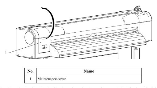
5. Move the print head section by hand to where the circumference of the Print head is visible.
